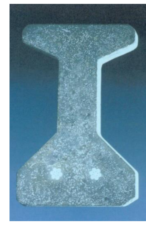
Tests of beams for Cattenom NPP cooling tower, 1997 – first design rules for EDF
