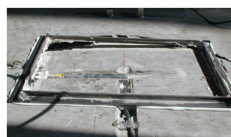
Direct anchor length identification in a re-bar pull-out test equipped with optic fiber BADIFOPS project, 2012
