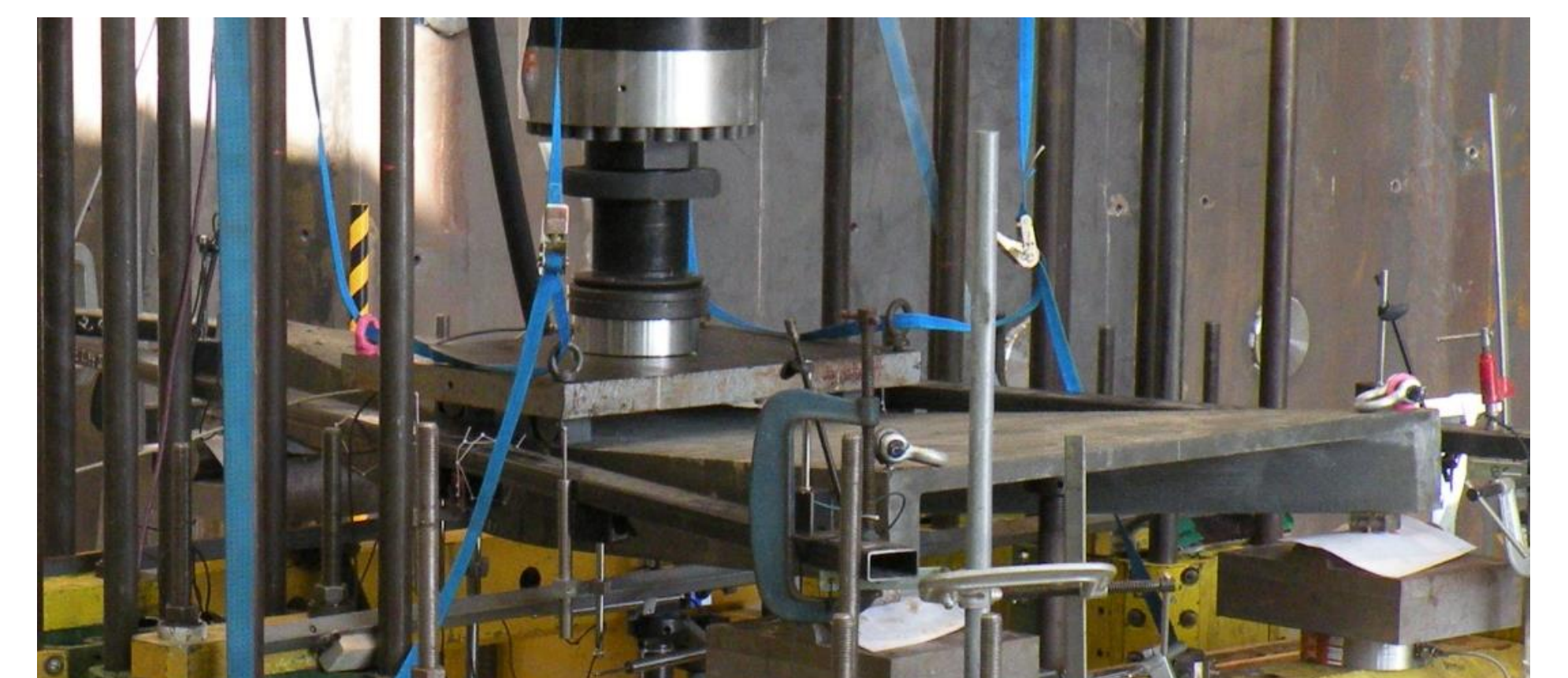
Ductility analysis for a two-reinforced ribbed thin UHPFRC triangle plate (following implication in Jean Bouin project), Guénet 2016
