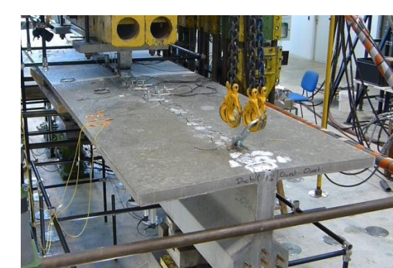
Shear tests on prestressed / reinforced beams for validating shear design provisions, 2009 - 2017
